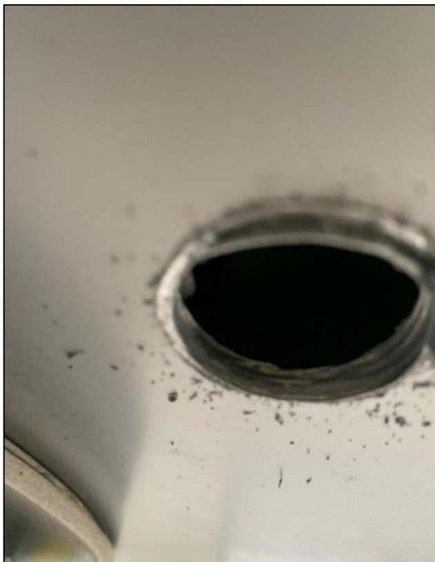
Photograph 2 – Sample of ACP cladding taken from the Awning on the Western Elevation
